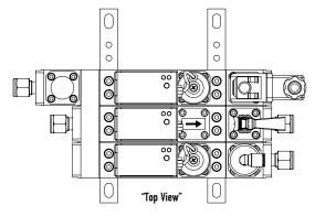
FLOW-SMS system by arranging functional modules viz. flow or pressure meters/controllers, valves and filters in combination with mixing chambers, adapter plates, mounting rails, etc. (see below example).
